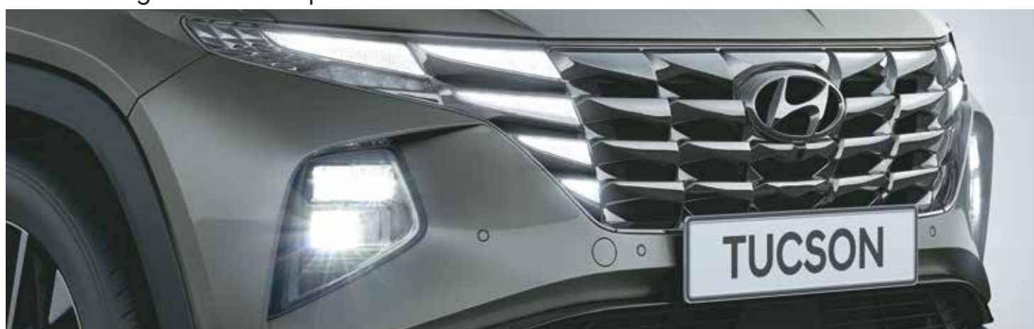
Dark chrome parametric front grille with parametric hidden LED DRLs, LED MFR headlamps & positioning lamps
